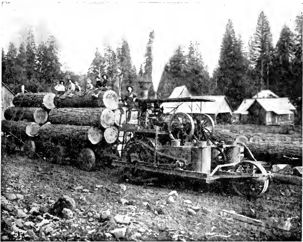
FIG. 58. — A Holt Three-wheeled Traction Engine hauling Sugar Pine Logs, California.
